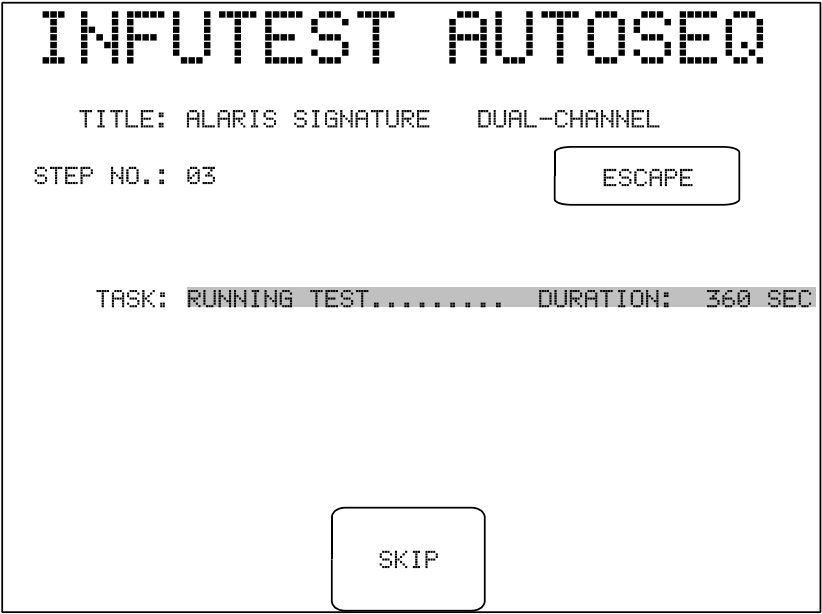
Figure 80: ES601 monitors Infutest status while Infutest tests the IV pump.
