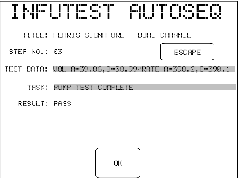
Figure 82: ES601 automatically passes or fails the final test results.
