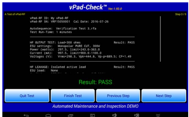
Figure 53 - ESU performance test results.
