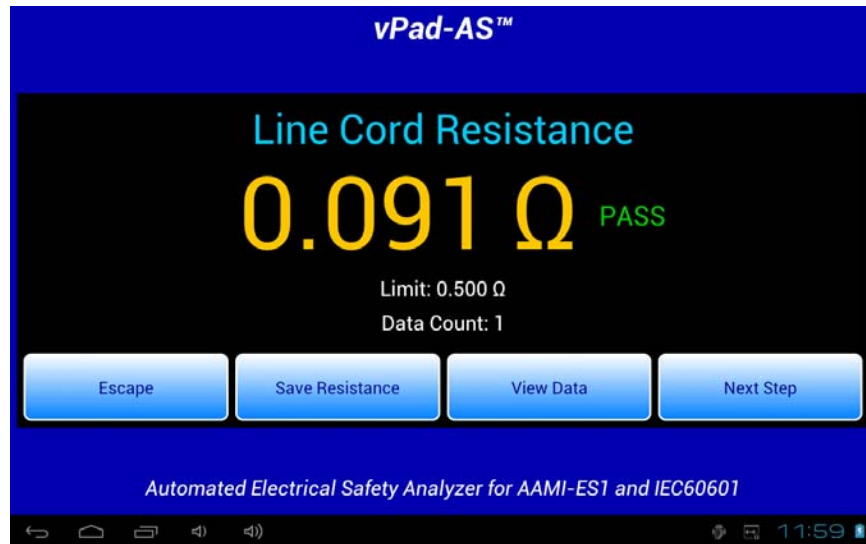
Figure 41 - Line cord resistance measurement.
