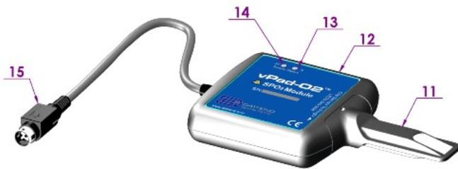
The vPad-O2 (**SpO2**) module is a pulse oximeter tester which connects to the **Base** module via a miniDIN8 connector. This module provides an artificial ‘finger’ containing light guides which convey light to or from pulse oximeter probes and sensors.
