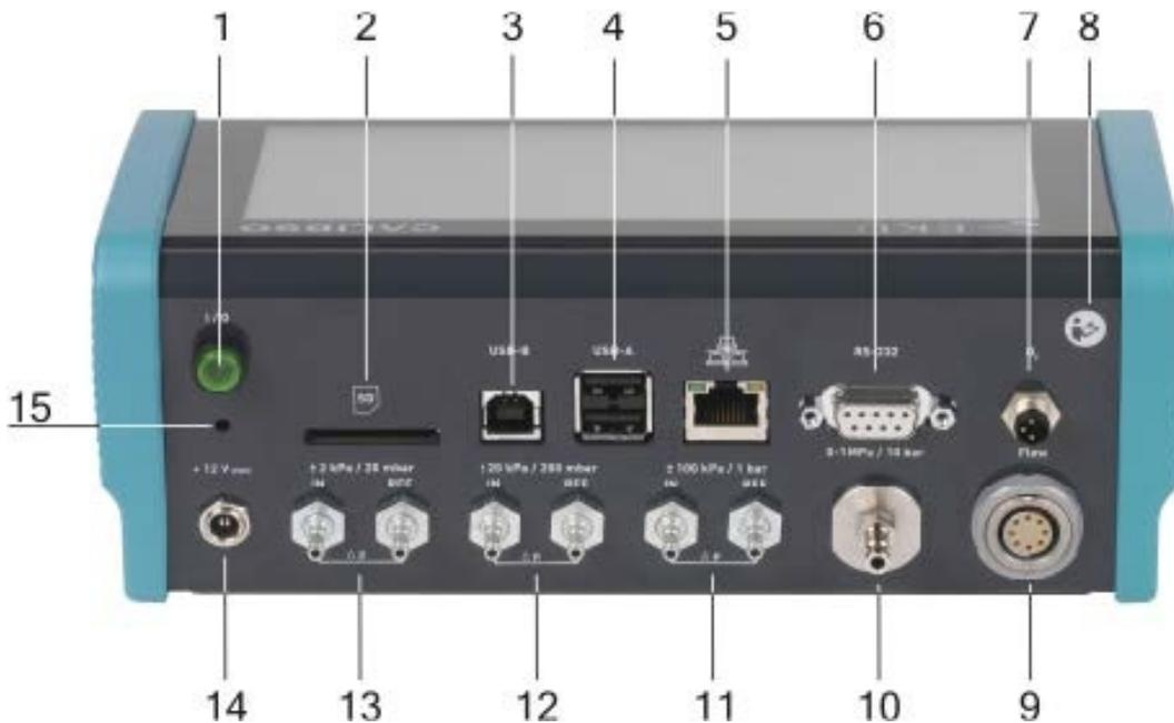
Figure 1 - venTest Base Unit Back Panel
