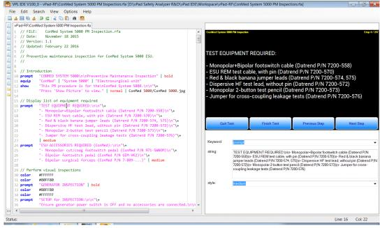
**Figure 14** - Editing a RFA file with the vPad Integrated Development Environment (IDE).
