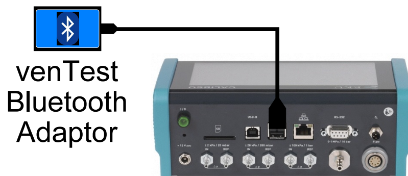
Figure 1 - Connection of adaptor 7400-116 to venTest USB.
