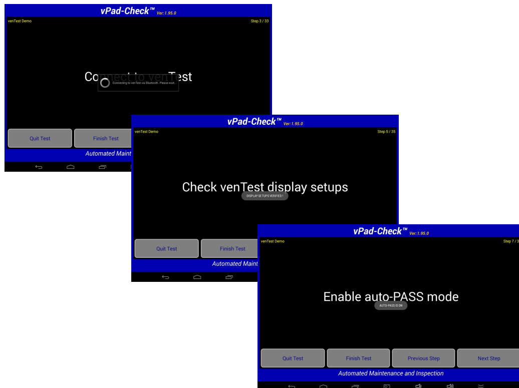
Figure 18 - Bluetooth connection, Display Setup verification, and enabling of test automation.
