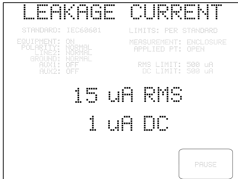
Figure 33 - Leakage current test in progress.
