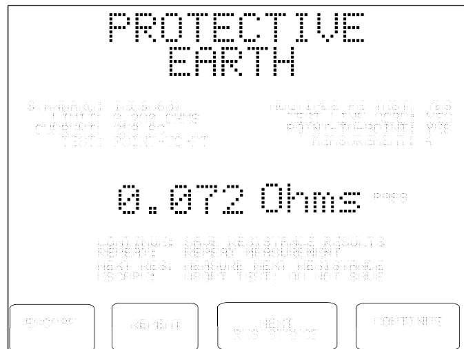
Figure 27 - Protective earth test result (multiple PE = "YES").
