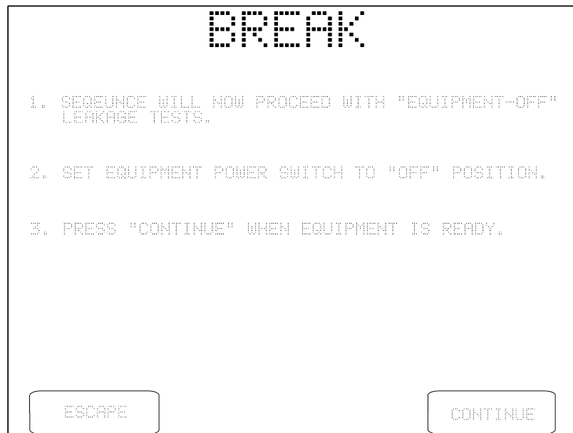
Figure 38 - Switch DUT to "OFF" for "DUT OFF" tests.
