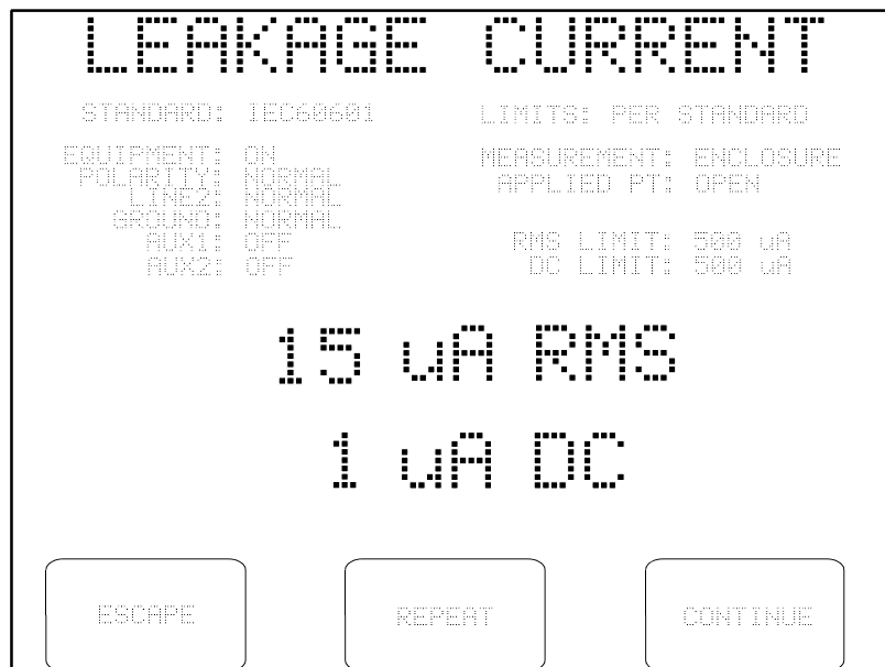
Figure 34 - Leakage test paused during sequence.
