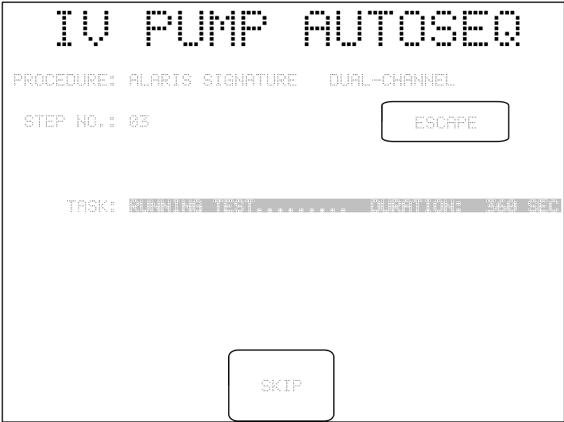
Figure 68: ES601 monitors Infutest status while Infutest tests the IV pump.
