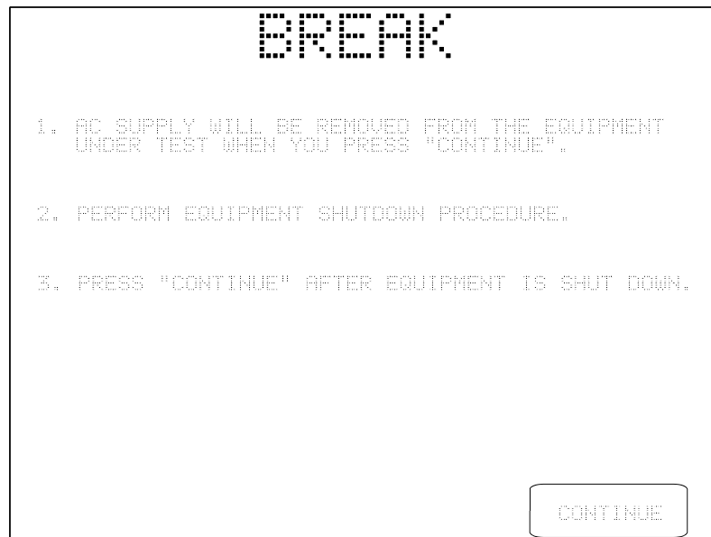
Figure 21 - Break if "STOP BEFORE..." system setting is "YES".
