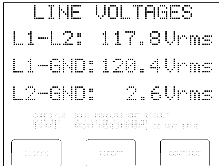
Figure 18 - Line voltage measurement results.
