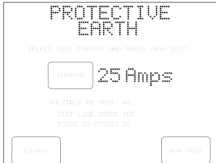
Figure 25 - Selection of test current (PETM option only).
