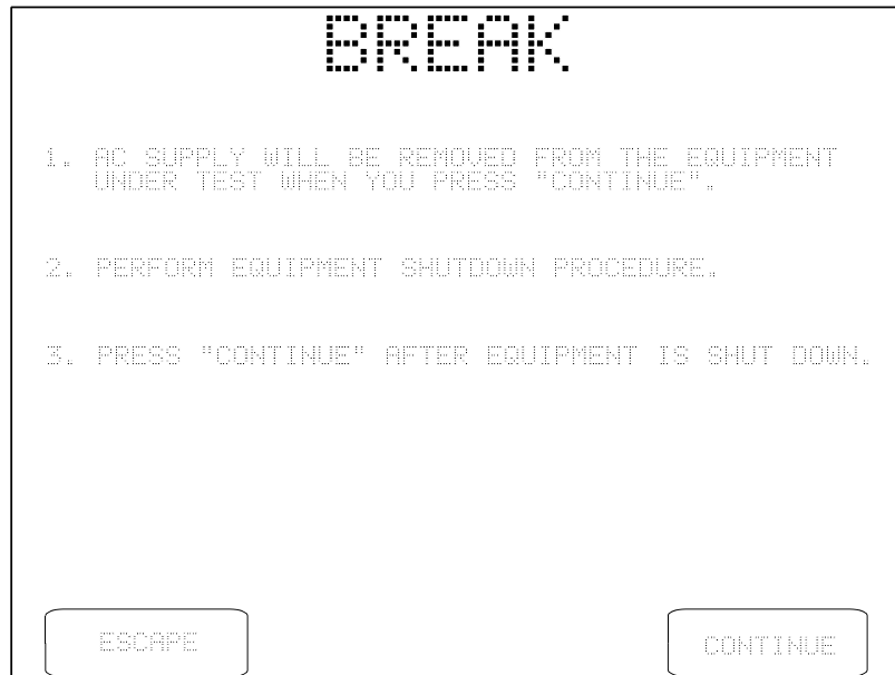
Figure 36 - Break if "STOP BEFORE..." is set to "YES".
