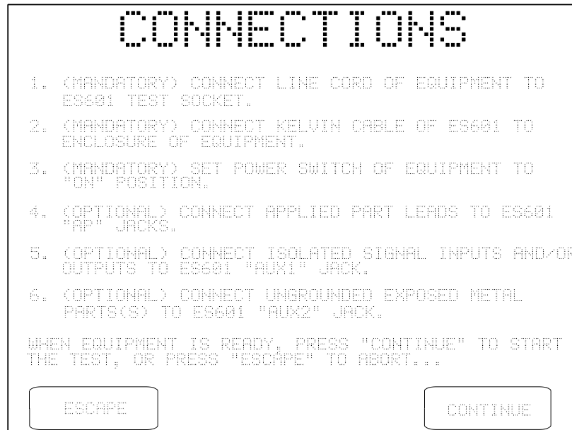
Figure 32 - DUT connection instructions for IEC60601 test.
