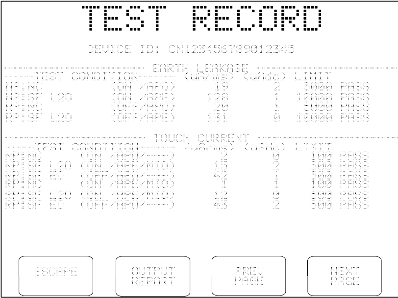
Figure 42 - Example of earth leakage and touch current results.
