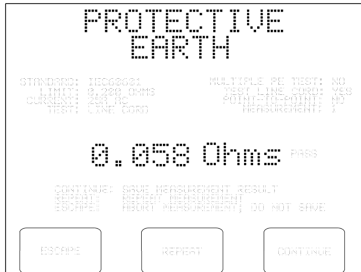
Figure 26 - Protective earth test result (multiple PE = "NO").
