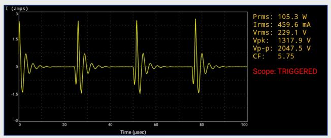
Figure 3: Screenshot of vPad-RF app displaying an ESU waveform.
