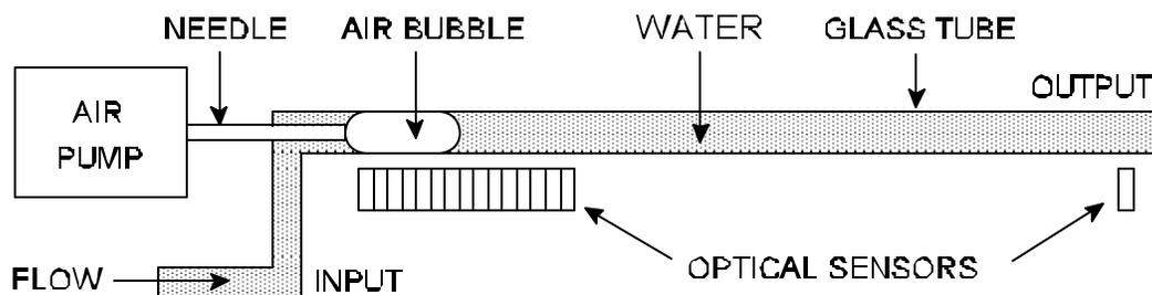
**FIG. 1 - Schematic of Infutest flow sensor.**
